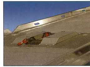
Low profile winch system allows flat alignment of upper and lower decks, permitting damage free loading/unloading of low profile vehicles.
