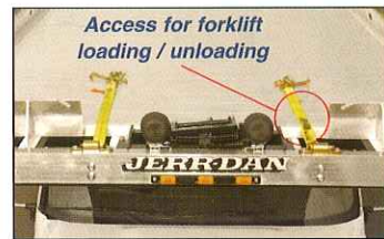
Access for forklift loading / unloading Upper deck winch release and hold-down straps are easily accessible through deck openings.
