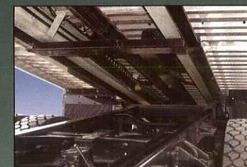
Dual state of the art hose & wiring cable carrier system protects hoses from crushing or kinking; high performance polymer slide pads provide greaseless long-life, operation.
