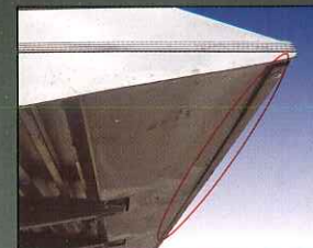
Pioneer Aluminum Carrier Approach Tip Wear Strip Jerr-Dan's exclusive stainless steel approach tip wear strip is designed to help you be the best, for a long time.
