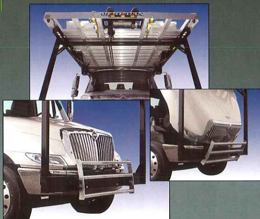
Upper deck is readily accessible through deck cut-outs and the three-rung step ladder on the front superstructure. Removable lock pins allow the ladder to tilt out for engine compartment access.
