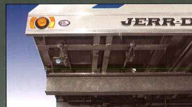
Dual remote winch releases mounted under deck for convenient operation of low-profile winches on lower deck.
