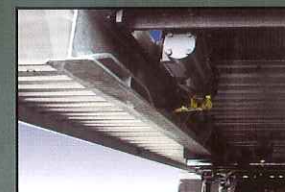
Exclusive Steelbeam Technology Hot-dipped galvanized steel longitudinal beams support the entire length of this new aluminum deck. Jerr-Dan's STEELBEAM technology securely joins both aluminum and steel for a lightweight, high strength, corrosion resistant structure.
