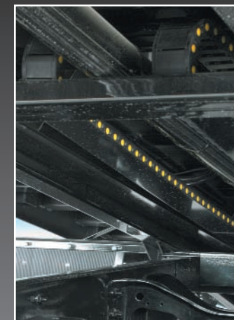
polymer slide pads provide greaseless long-life, operation.
