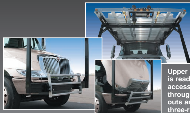
Upper deck is readily accessible through cut-outs and the three-rung step ladder on the front superstructure. Removable lock pins allow the ladder to tilt out for engine compartment access.
