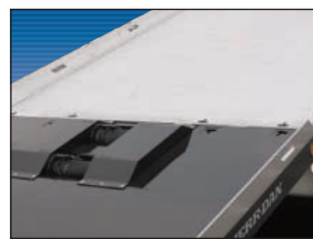
Low profile winch system allows flat alignment of upper and lower decks, permitting damage free loading/unloading of low profile vehicles.
