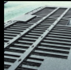
8" Crossmember Spacing (Dual Center Keyslots, Rubrail Keyslots and Wheel Wells Shown)
