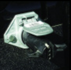
7-Way Plug with Adapter / 7-Round to 4-Flat and 7-Round to 6-Round (Standard with 10 and 15 Ton Tow Options)
